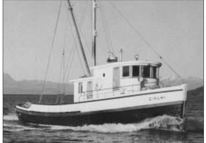
The Gikumi was launched with a 190-hp Atlas Imperial diesel which Fred Wastell replaced with a Nissan V-8 diesel in 1974. The latest engine, installed by Jim Borrowman in 1997, is a Caterpillar 3406B which provides 8-9 knots at 900-1000 rpm.
